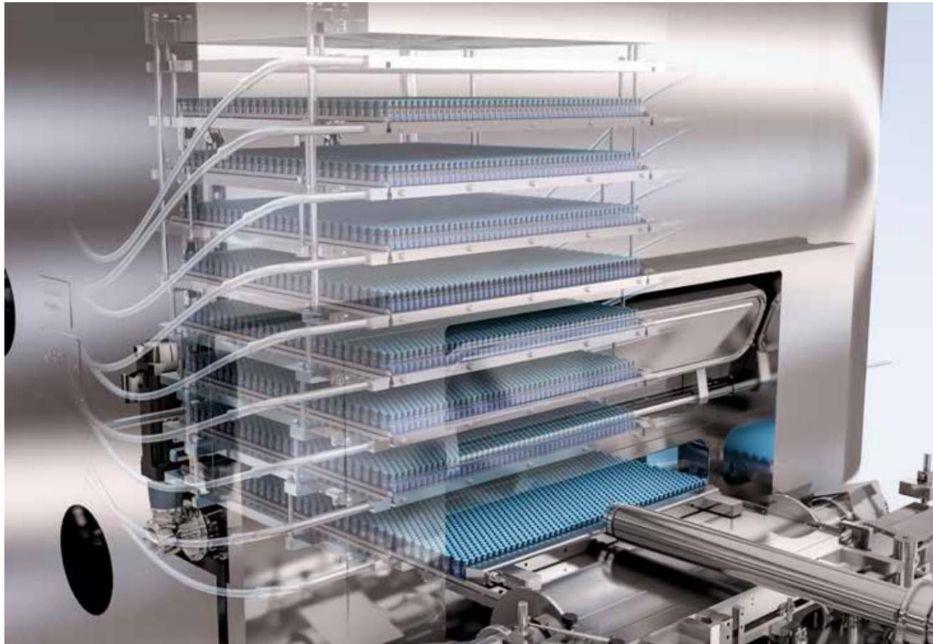
^ The integrated freeze dryer is accompanied by an automatic loading and unloading system that slides the vials into the freeze dryer row by row. The vials are separated again during unloading.
