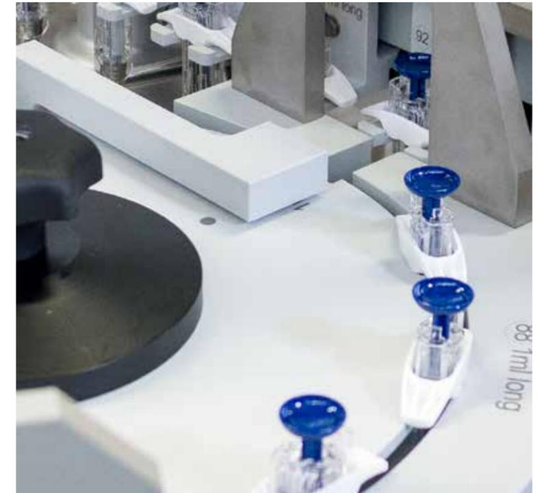
At USV India, a second Optima system assembles safety devices. The syringes are also labelled.
