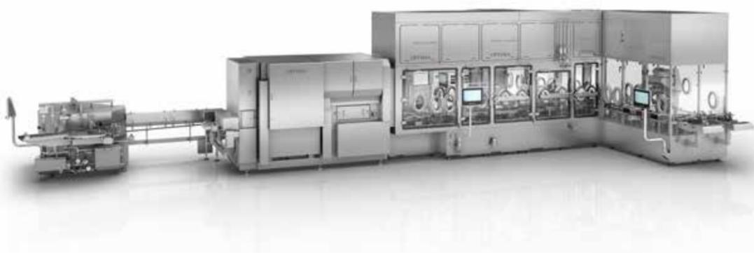
At Catalent, the OPTIMA VFVM 18000 filling and closing machine is used. The complete filling line handles washing, sterilizing, filling and closing of vials under isolator.
