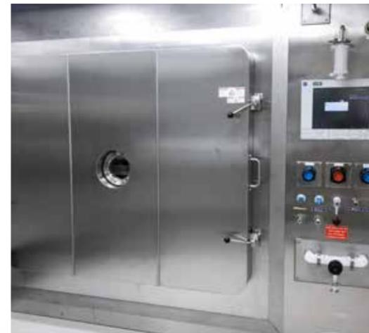
The freeze dryer chamber with door can be seen. Bachem is now using freeze dryers from Optima for the first time.
