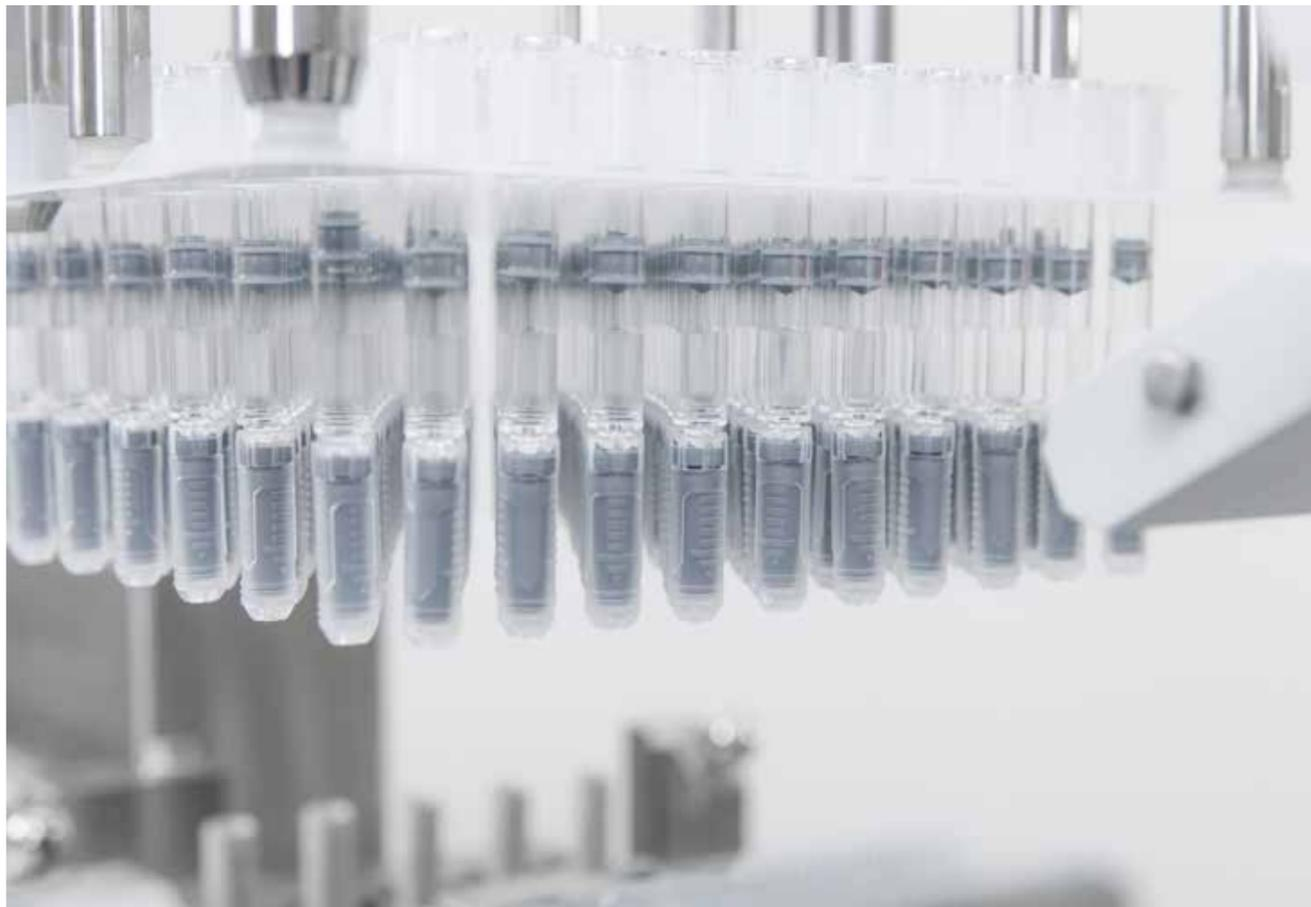
^ The pharmaceutical company USV in India placed the awarding of the contract on the flexibility of the filling solution. The OPTIMA SV125 currently processes nested ready-to-use syringes in the formats 1 ml long, 3 ml (in different formats) and 5 ml as well as cartridges.
