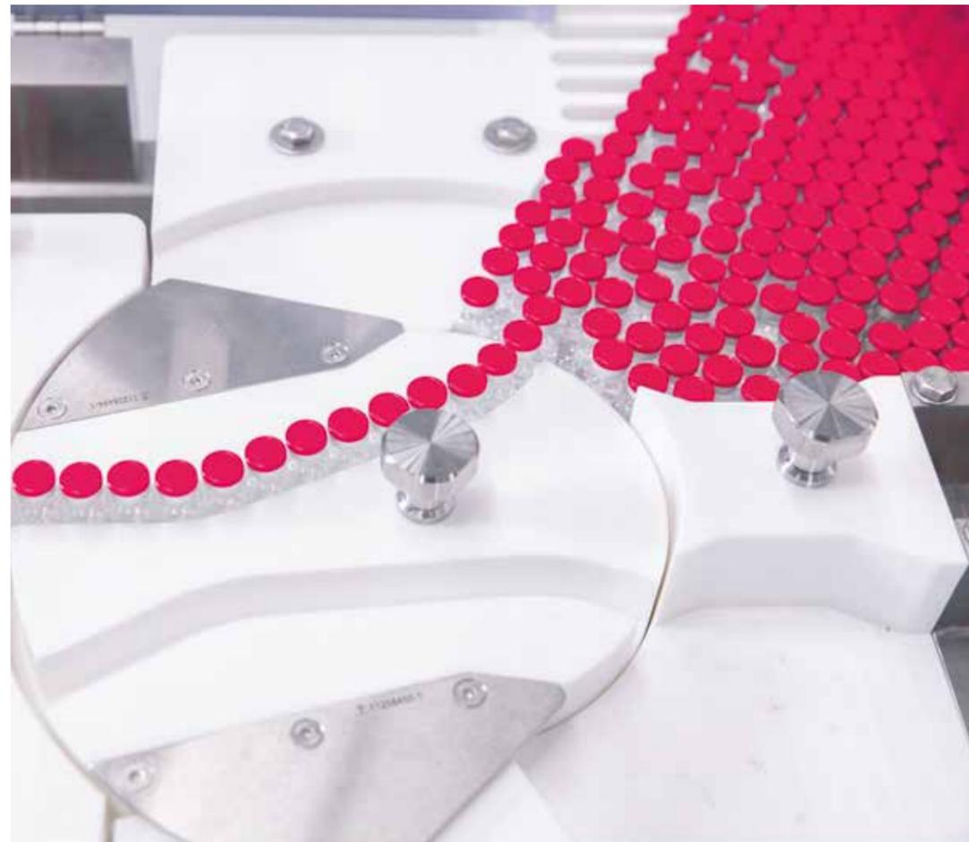
Vials filled with vaccines and tested are lined up and compactly grouped with a tray loader.
