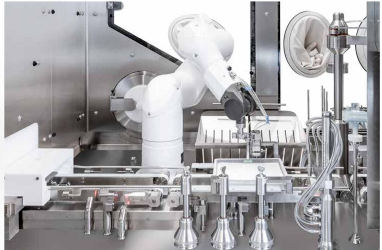
^ The Tyvek Removal Robot removes the sealed film from the nest before separating the containers inside.
