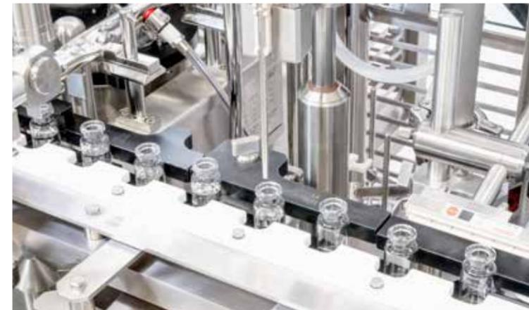
The new, fully automated vial filling and closing line with RABS started operating at Biovian in early 2021. It can process a range of vial sizes up to a batch size of 10,000 vials. <
