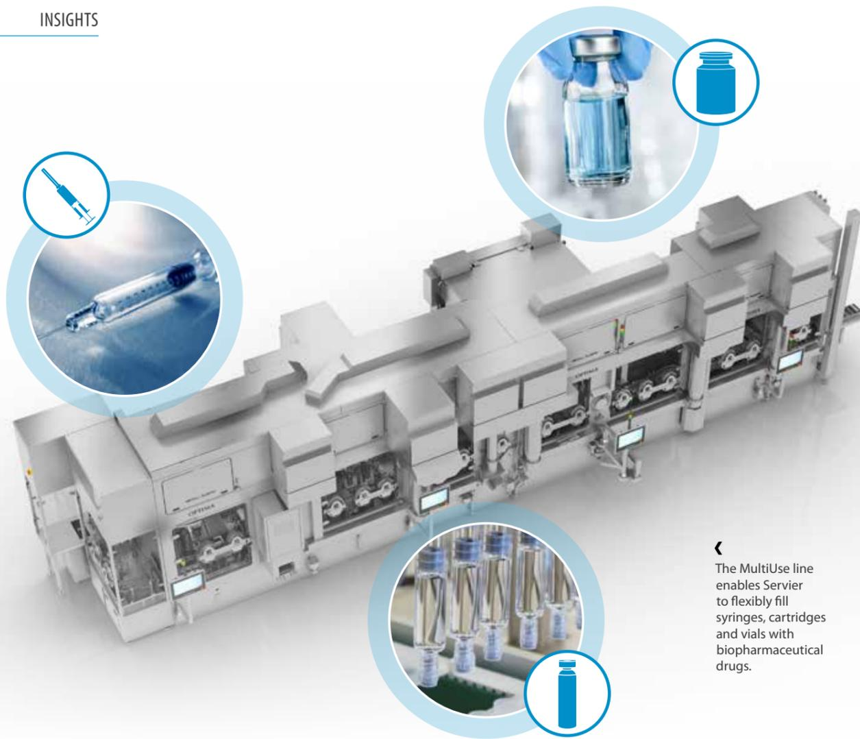
◀ The MultiUse line enables Servier to flexibly fill syringes, cartridges and vials with biopharmaceutical drugs.
