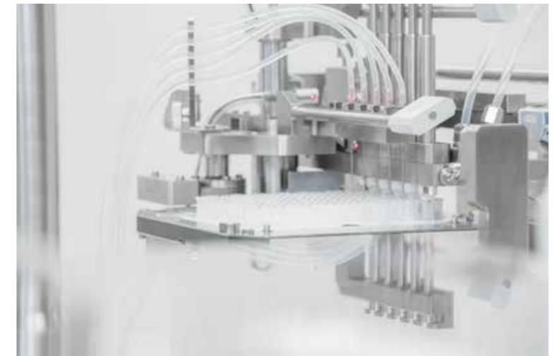
^ As a standard dosing system, USV uses rotary piston pumps in the OPTIMA SV125. In addition, USV can fall back on a five-position peristaltic pump system at any time.
