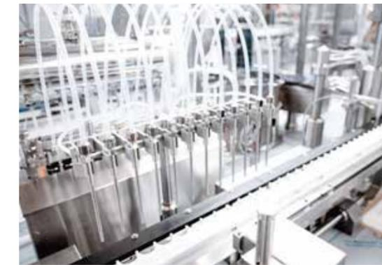
◀ By combining different processes, the line masters the dosing of four media with very different properties – from spray dosing of a liquid to the addition of the resin-like reagent.
