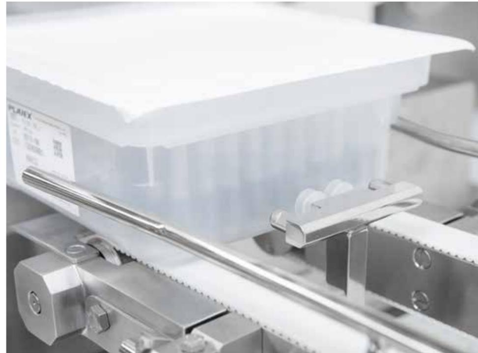
An OPTIMA TRR Tyvek Removal Robot will soon be peeling off the protective film.
