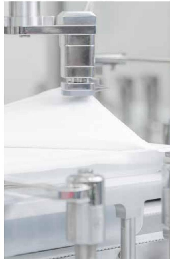
^ The removal of the sealed foil of the tub and the removal of the Tyvek cover is done fully automatically.
