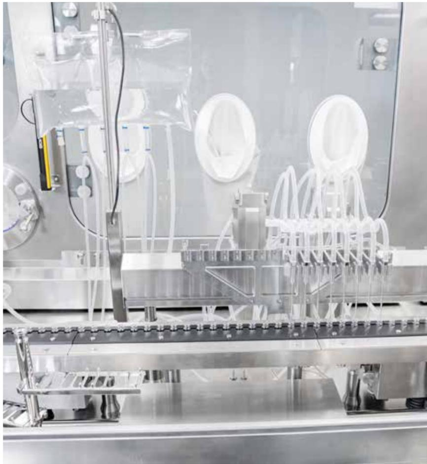
High speed, precision filling: Up to 24,000 vials per hour are processed by the system. 100 percent of the containers are inspected by an in-process control.
