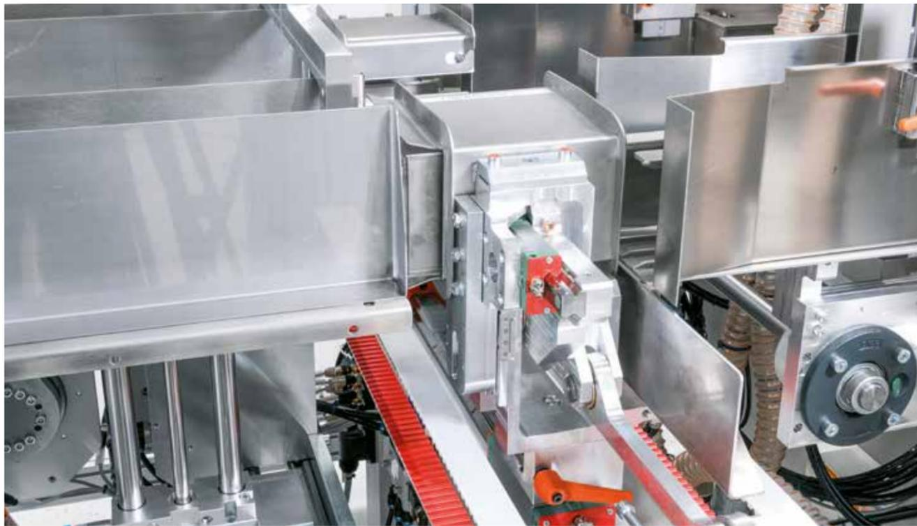
^ In the pivoting cassette the products are turned as required. Together with the new turnbox (see image on page 23) all product alignments can be achieved – without module changeover.
