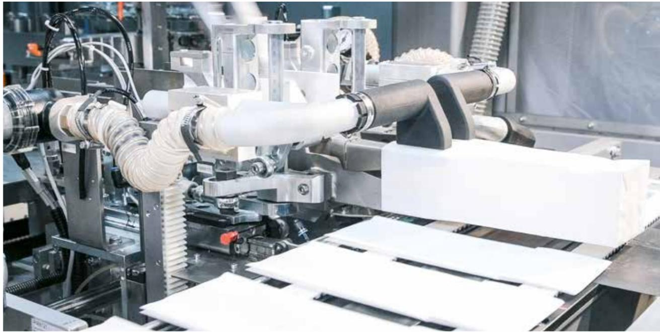
^ The feminine hygiene products are pushed at high speed through the shuttle to the opened pack.
