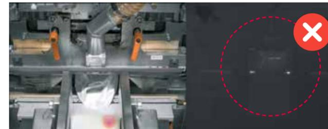
◀ The thermal imaging camera (right) allows differences (top to bottom image) in the weld to be detected even at high speed.
